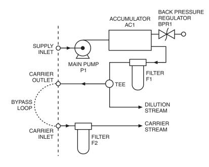
Figure 8: Diagram of configuration 3
