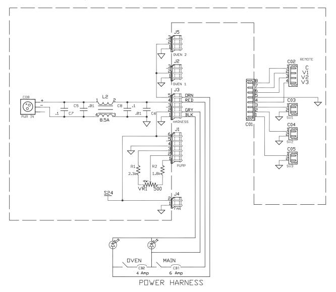
**Figure 11:** Model 230 electrical schematic (*Refer to page 37 for Electronic Flow Control option*)
