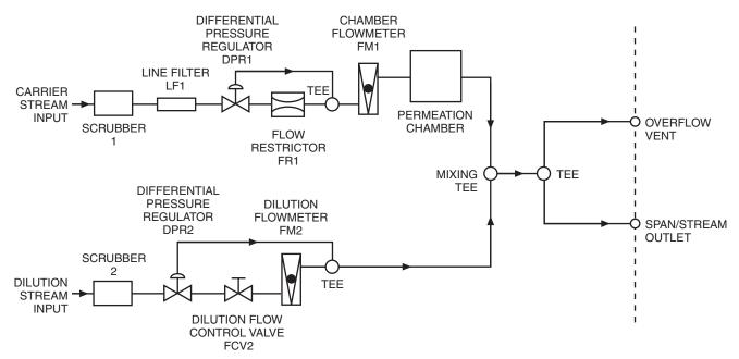
Figure 1a: Model 230 standard plumbing schematic
