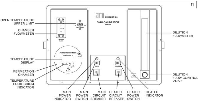
Figure 3: Model 230 front panel controls and indicators (Refer to page 36 for Electronic Flow Control option)
